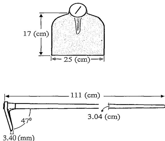
**Figure 1.** Specifications of the hoe designs used for weed control on hillsides.
